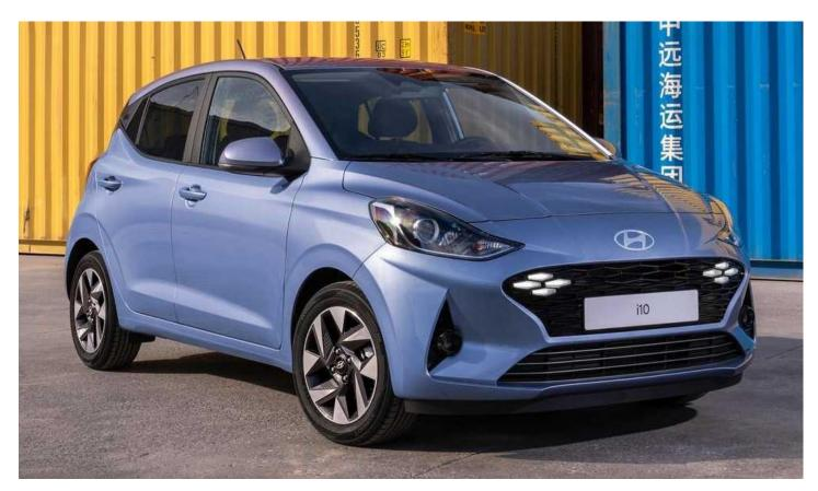
Length: 3,670mm Width: 1,680mm Height: 1,480mm Wheelbase: 2,425mm Fuel Tank: 36( $\ell$ ) Luggage Compartment: 252lt. (1,050 lt. with rear seats down).
