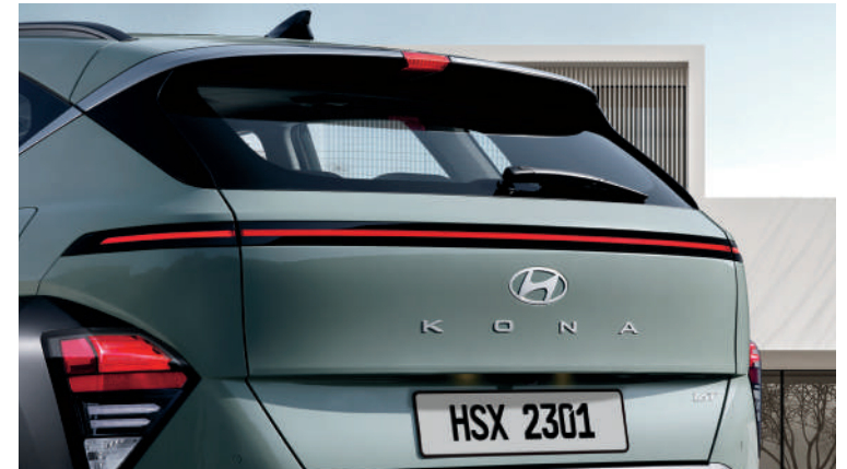
Spoiler Integrated HMSL, rear seamless horizon lamp LED brake lamps, LED turn signal lamps
