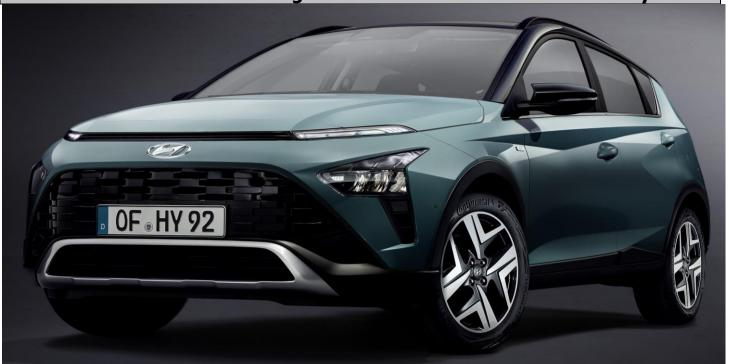
Length:4,180mm Width:1,775mm Height:1,500mm Wheelbase:2,580mm Fuel Tank: 40(ℓ) Boot space:401lt. (1.205 lt. with rear seats down) Ground Clearance: 16,50cm (16") - 18,30cm (17")
