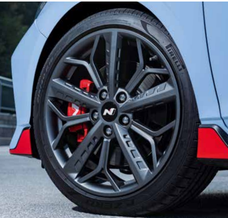
The bespoke 18-inch alloy wheels with a grey matte finish and N-branded brake callipers highlight the all-new i20 N's high-performance credentials. They are paired with Pirelli P-Zero ultra-high-performance tyres, which sport the initials "HN" to indicate that they have been specially developed for Hyundai N.
