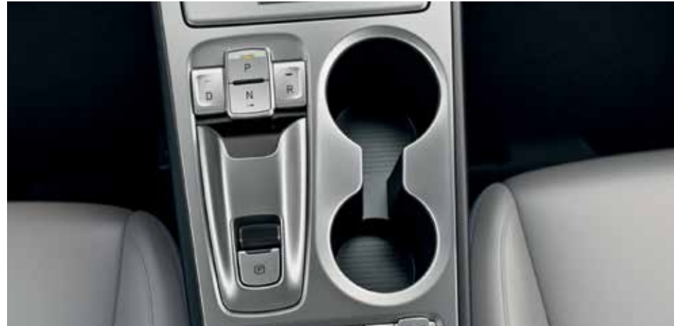
Button type shift-by-wire. Everything you need, right at your fingertips – switch between drive, neutral, reverse and park by simply using the buttons conveniently located within the centre console. The electric parking brake can be found here as well.
