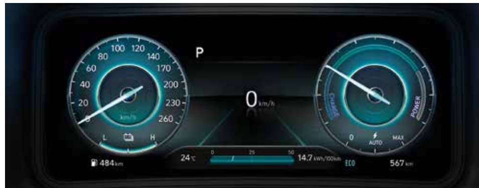
New 10.25" fully digital cluster. One glance is all it takes to see how your driving style is influencing your driving range. Its colour schemes change depending on which drive mode is selected. Choose from Comfort, Eco or Sport. There is also an additional Cube interface design for a different look
