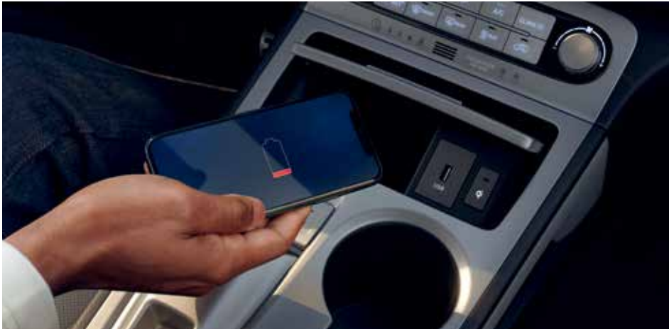
Wireless charging. A wireless charging tray is located conveniently in the centre console. Now you can easily and quickly charge a compatible Qi-enabled smartphone without the hassle of having to plug it in.
