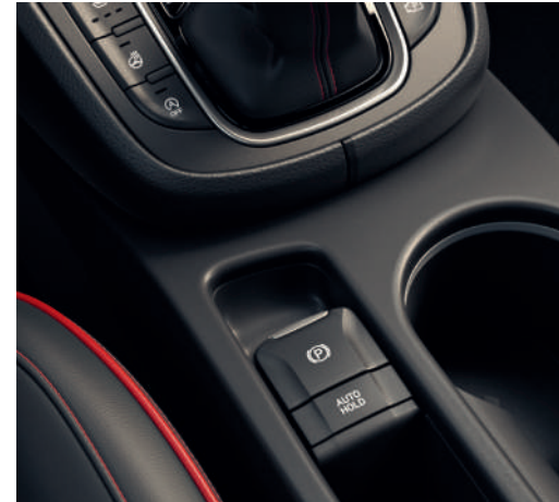
Electronic parking brake. Enjoy finger-tip control. An easy-to-use button activates or deactivates the electronic parking brake. The clever Auto Hold feature keeps your vehicle at a complete stop without you having to keep your foot on the brake pedal.
