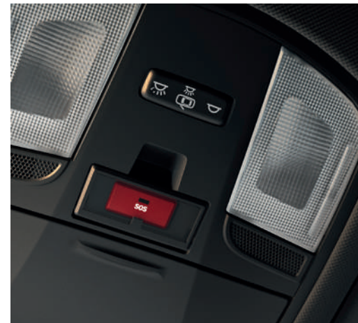
E-call button. This feature automatically calls emergency services if you're in an accident and the airbags deploy. You can also push the SOS button for emergency assistance at any time.
